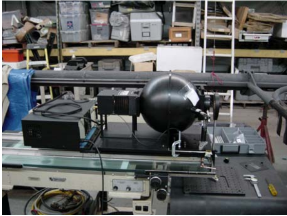
Setup with OL455 sphere and fiber optic jig
