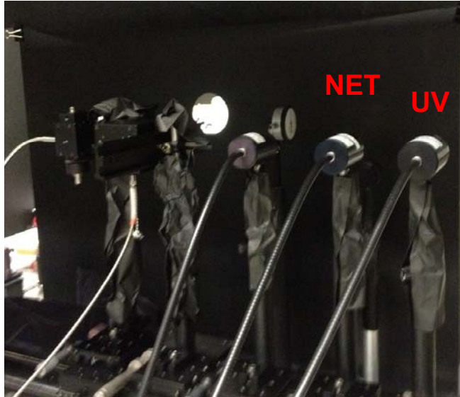
Four CAS' and one SEI on an x,z translation stage
