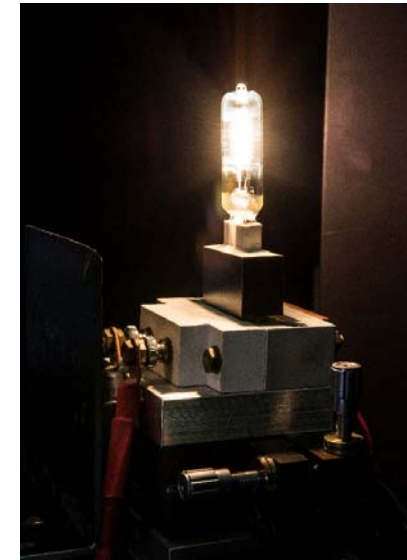
An 1000 W FEL spectral irradiance standard lamp is 50 cm away
