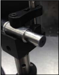
Lu fiber bundle, input side (10 mm diam)
