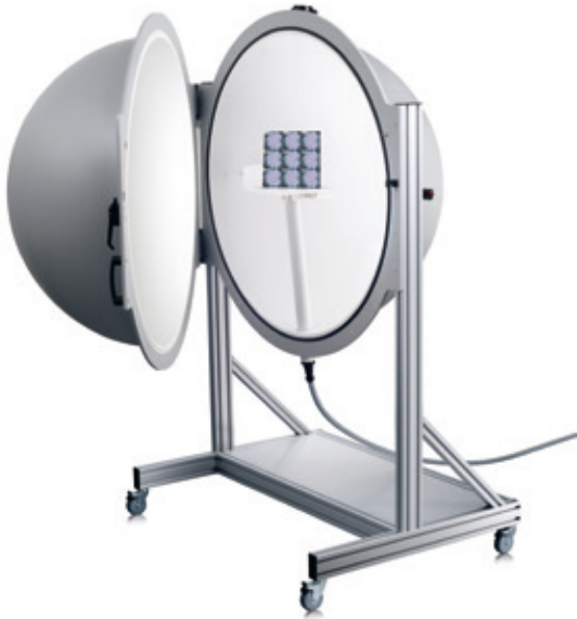
The ISP 1000 integrating sphere with 1 m diameter
