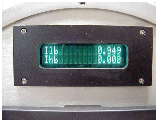
Figure 3. Ilb Low beam (top) and Ihb High beam (bottom) lamp currents. Note here only the low beams are active.
