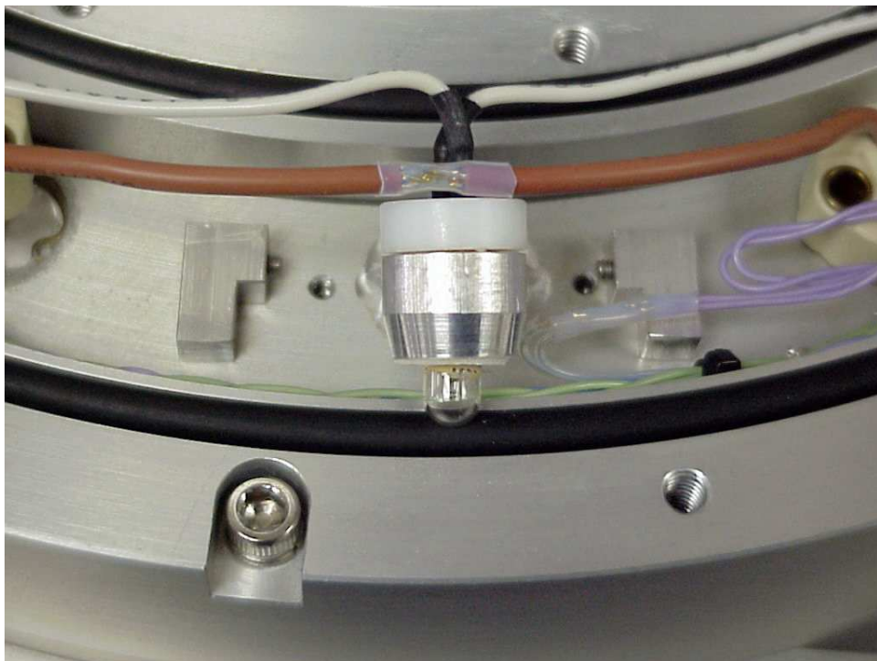
Figure 13. Smaller socket removed, bulb in socket, side clamps at left and right.
