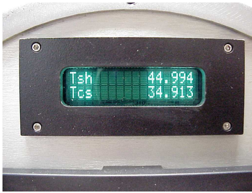
Figure 6. Tsh temperature of shunts (in °C, top) and the Tcs lamp case (bottom). The lamp temperature measurement is made at the lamp rings, which is close to the air temperature inside the optical integrating cavity that houses the lamps.
