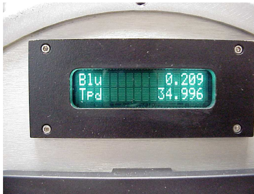
Figure 5. Blue monitor detector output (top) and Tpd detector thermoelectric cooler temperature, in °C (bottom).
