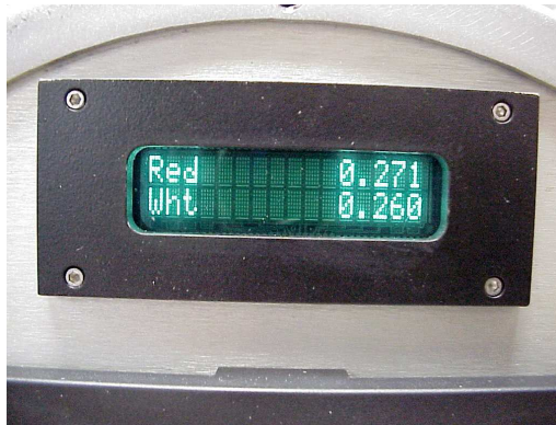
Figure 4. Red (top) and unfiltered/white (bottom) optical monitor outputs.
