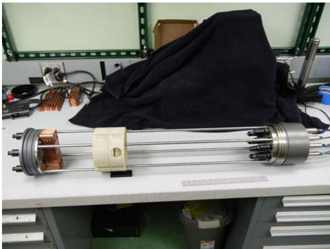
Internal housing frame (outer tube removed, MIFS radiometer not installed)
