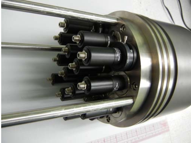
Spectrograph side, 14 collimators with iris
